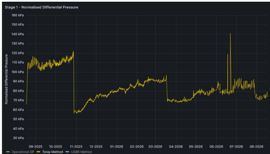
Figure 1: Normalised differential pressure of the RO membranes at Hawker WTP.
