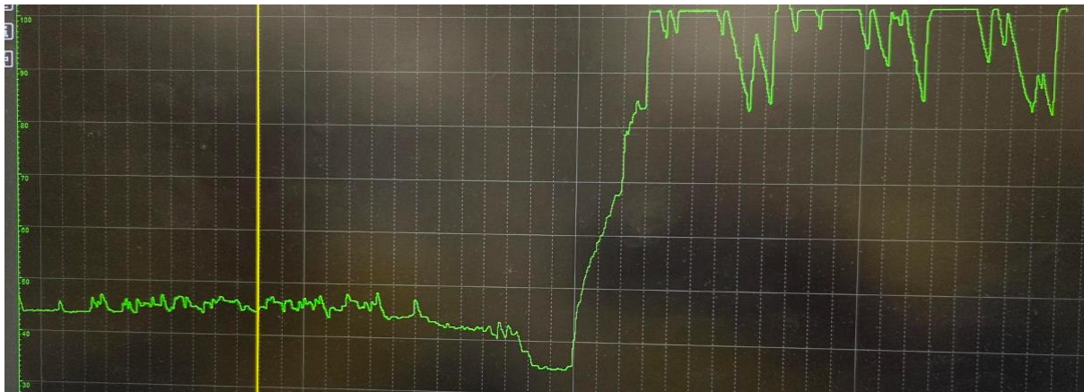
Figure 6 Overhead radar trends for hopper 2 with AirSweep® upon initial installation
