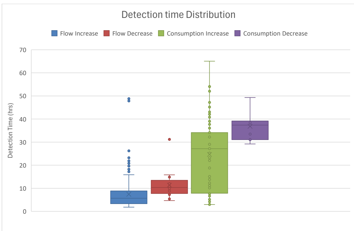
Figure 4 Detection Time Distribution for flow and consumption events
