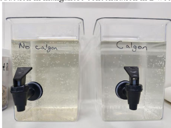
Figure 3 – Comparison of Jars after 2 weeks post-dose (Left: without Calgon; Right: Calgon dosed)
