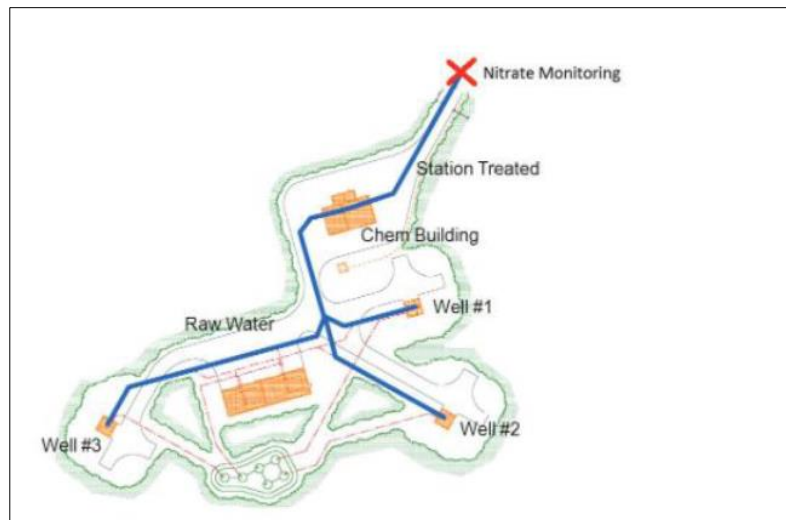
Figure 1: One of the many sites the utility extracts groundwater from. At this site, the water is drawn from three wells, one of which has a high concentration of nitrates, blended, chlorinated in Chem Building, and monitored for pH, residual chlorine and nitrates before being pumped to the consumers.
