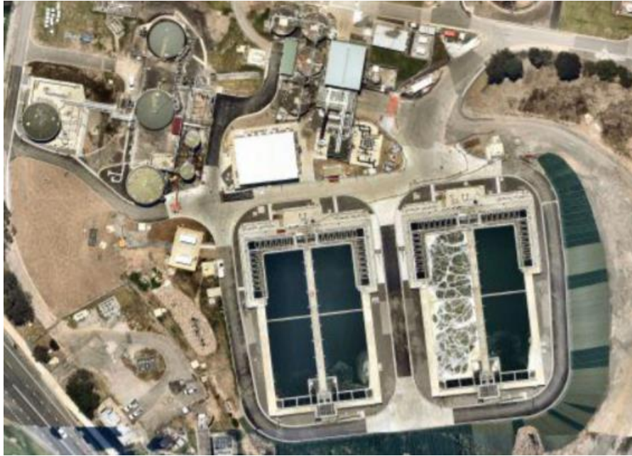
West Camden WRP, New South Wales. Upgraded with dual MBRs to replace IDALs - commissioned 2025
