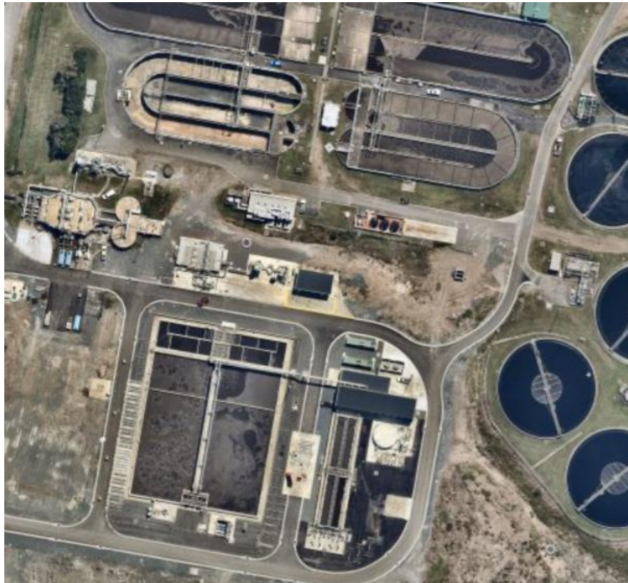
Loganholme WWTP, Queensland. MBR upgrade to augment existing oxidation ditch plant
