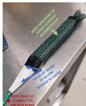
Figure 2: "Torpedo" passive sampler developed by Dave McCarthy (Monash University)
