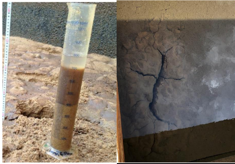
Figure 5: Solids retention test & media surface cracking
