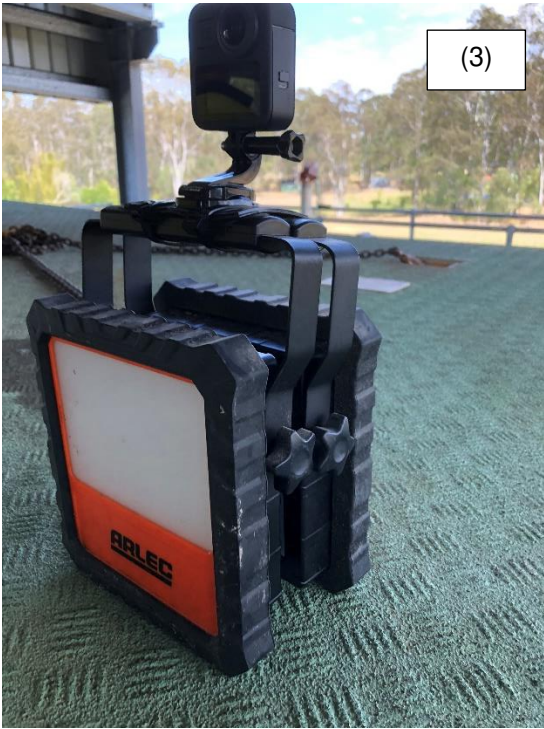
Figure 3: A Go-Pro 360 camera was used to inspect the lift station's wet well where conventional access is extremely difficult
