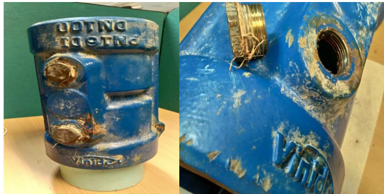
Figure 4 – Internal corrosion from the ReadyTap fitting
