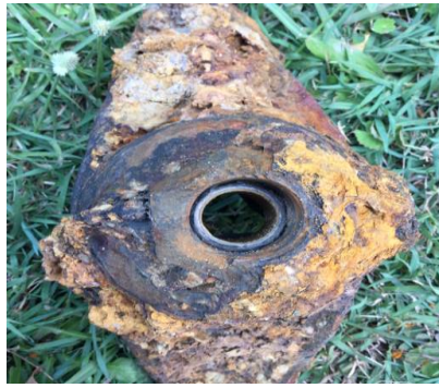
Figure 3 – Corrosion issue on steel tapping band
