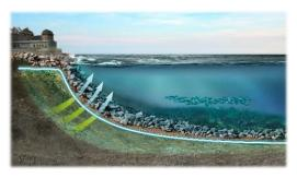
This application is the most complex and subject to site specific variations. In this case there is contaminated water or semi-liquid sediment that needs to be isolated, reducing PFAS spread. Geocomposites are nearly always the material of choice here. Geomembranes are problematic in that they commonly float/are buoyant in water, and those materials that do have negative buoyancy require anchoring to resist the
