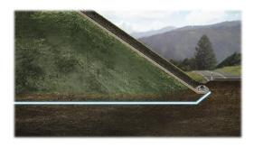
In this situation, the contaminated area is not moved, rather a cap or umbrella is placed over the area to provide a barrier to water intrusion and the resulting spread of PFASs into groundwater. In this case, the goal is to reduce or eliminate water moving into the contaminated soils. This is not a remediation, more of an isolation. Geomembrane is the common material of choice and is primarily selected for the ability to keep
