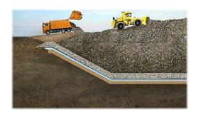
In this situation, materials are being moved to a location and installation designed to hold the contaminated soils for a long period of time. This movement is planned, in advance and a geotechnical barrier is installed to provide this containment for decades, or even centuries. This is the "Ziplock bag / baggie" option with barrier above and below the contaminated soils. It is usually used for highly contaminated materials due to the expense of
