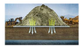
This application is when materials are to be stored on a long-term, but non-permeant basis. An example is PFAS contaminated soils being temporarily removed from a site during works. These soils would be stored on a pad, to prevent groundwater contamination and eventually returned to the site or moved to a permeant disposal location. For this situation, a geocomposite material is likely the best option – this protects against
