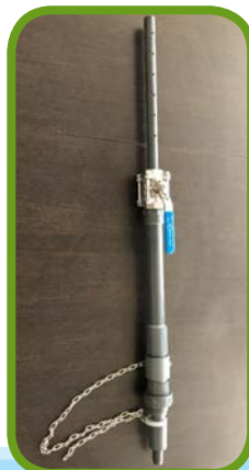
Perforated dosing lance retracted.
