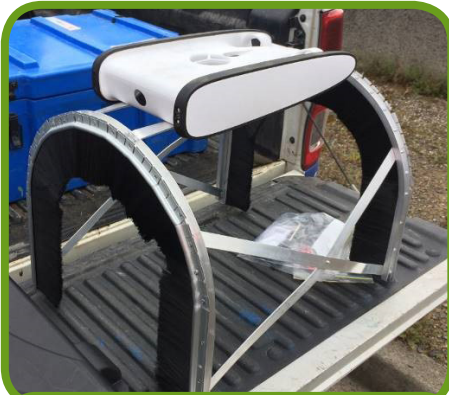
The brush arrangement powered by the ROV.
