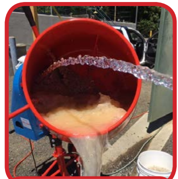
Pre-washed media being washed to clean.
