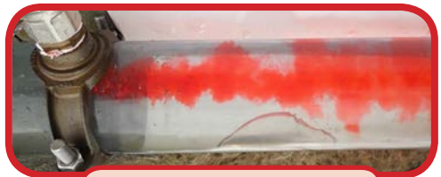
Mid stream dosing lance (traditional dosing) in the test rig.
