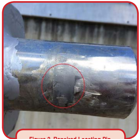
Figure 2. Repaired Locating Pin
