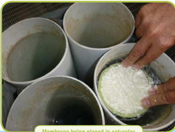
Membrane being placed in saturator
