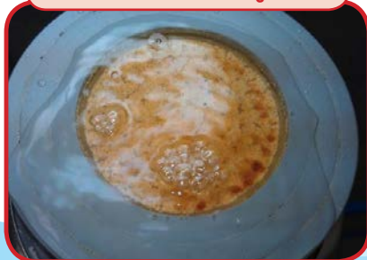
Membranes in test rig - false flow due to air ingress
