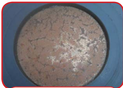
Membranes in test rig - false flow due to air ingress
