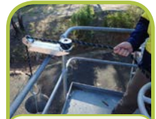
Lowering with rope wrapped as a brake
