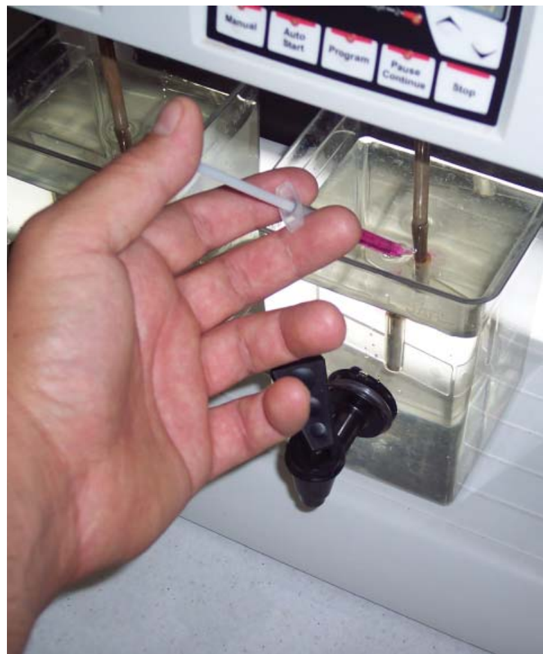
▼ Jar testing Potassium Permanganate doses.
