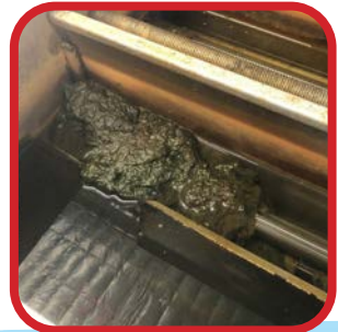
Clarifier outlet filter baskets and UV system blocked up by solids build
