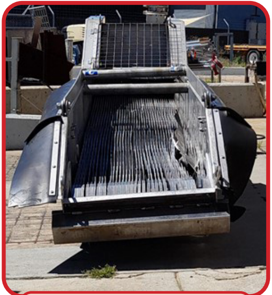
Damage to the existing step screen
