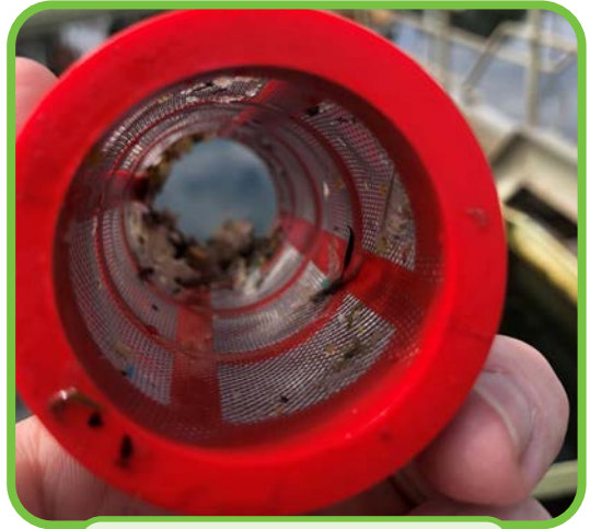
Inline filter during weekly inspection
