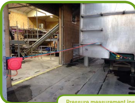
Pressure measurement installation to measure the amount of sludge loaded into trailers.
