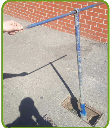
Valve key on top of the stoptap removal key
