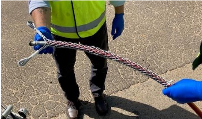
Figure 6. Hose restraint connection shackled to a HCB hose reel
