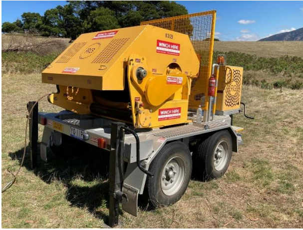
Figure 2: Cable Winching Trailer located at Downstream End (9t Rating)
