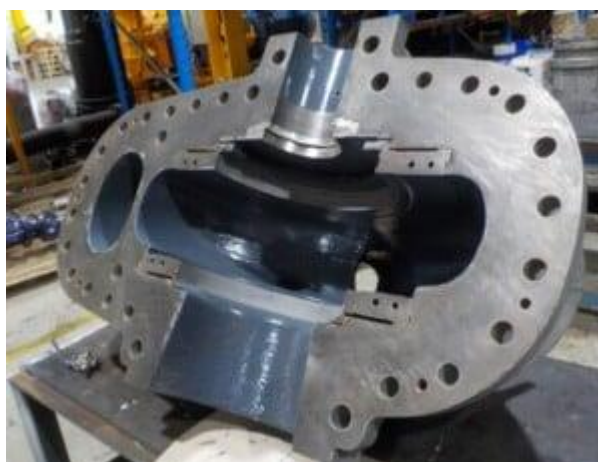
Figure 9: Pump casing repair and coating process showing machined wear ring locations and ARC ceramic coating applied.
