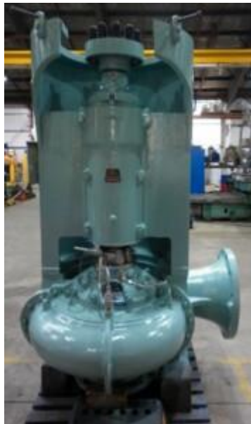
Figure 5: Vertical Sewage pump upgraded during overhaul with Chesterton 442 split seal, EnviroSeal SpiralTrac™ and Chesterton ARC ceramic coating
