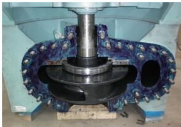
Figure 8: Pump casing repair and coating process showing machined wear ring locations and ARC ceramic coating applied.
