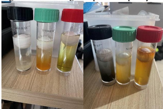
Figure 5 showing BART Kit after day 1 on the left and Day 8 on the right of a water bore. After Day 8 photo on the right reaction to Sulphate Reducing Bacteria SRB (Black Lid)
