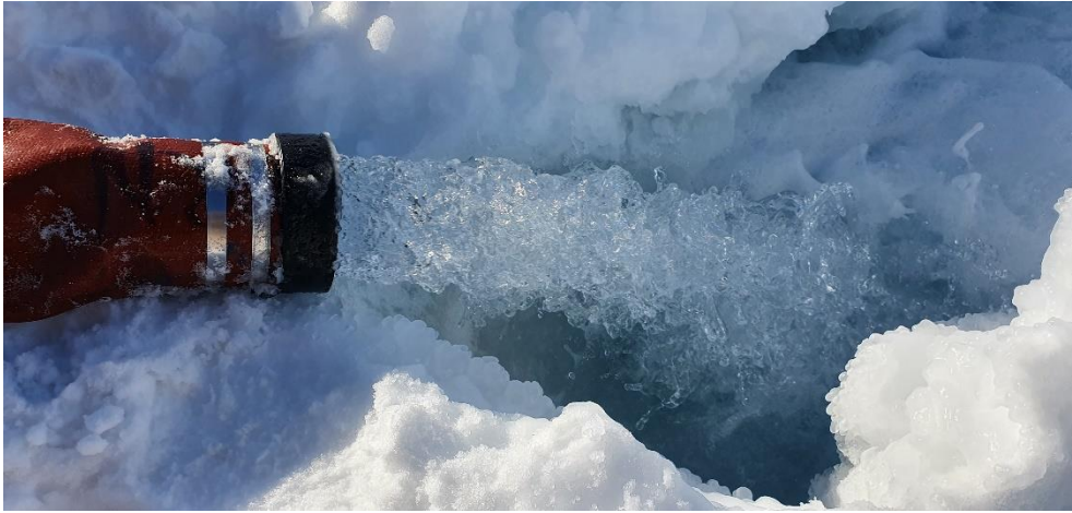
Figure 3: Pumped water exiting layflat hose as an ice/liquid mixture
