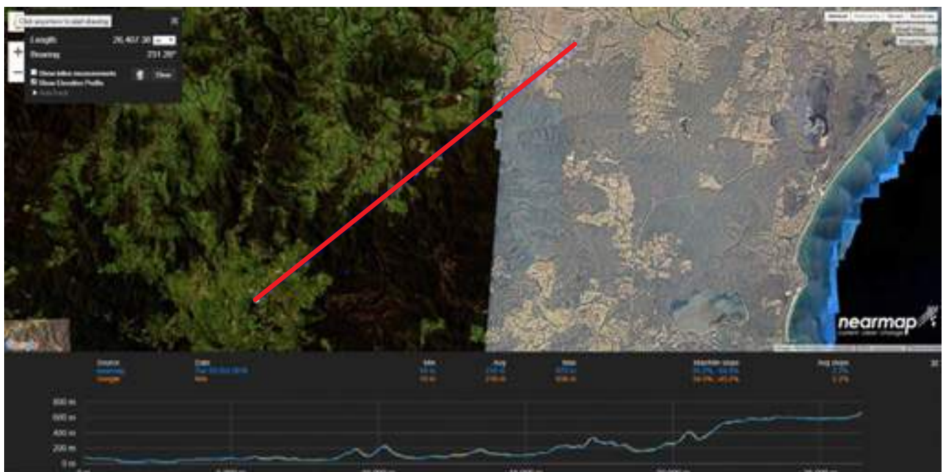
Figure 4. Signal path from Wauchope to Comboyne WTP.
