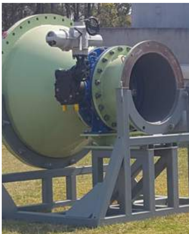
Figure 2. The photo on the left shows the newly developed solution sitting on the delivery stand (and what will be the future storage stand for the temporary valve once removed after the GKILR is re-installed). The photo shows the smaller inlet (1060 mm) flange, the new valve (blue) with gearbox (black) and Rotork actuator (grey) mounted, and also shows the downstream (1910 mm) flange that was engineered to replace the original bell shape of the GKILR. The photo on the right shows the solution being installed in place of the GKILR.
