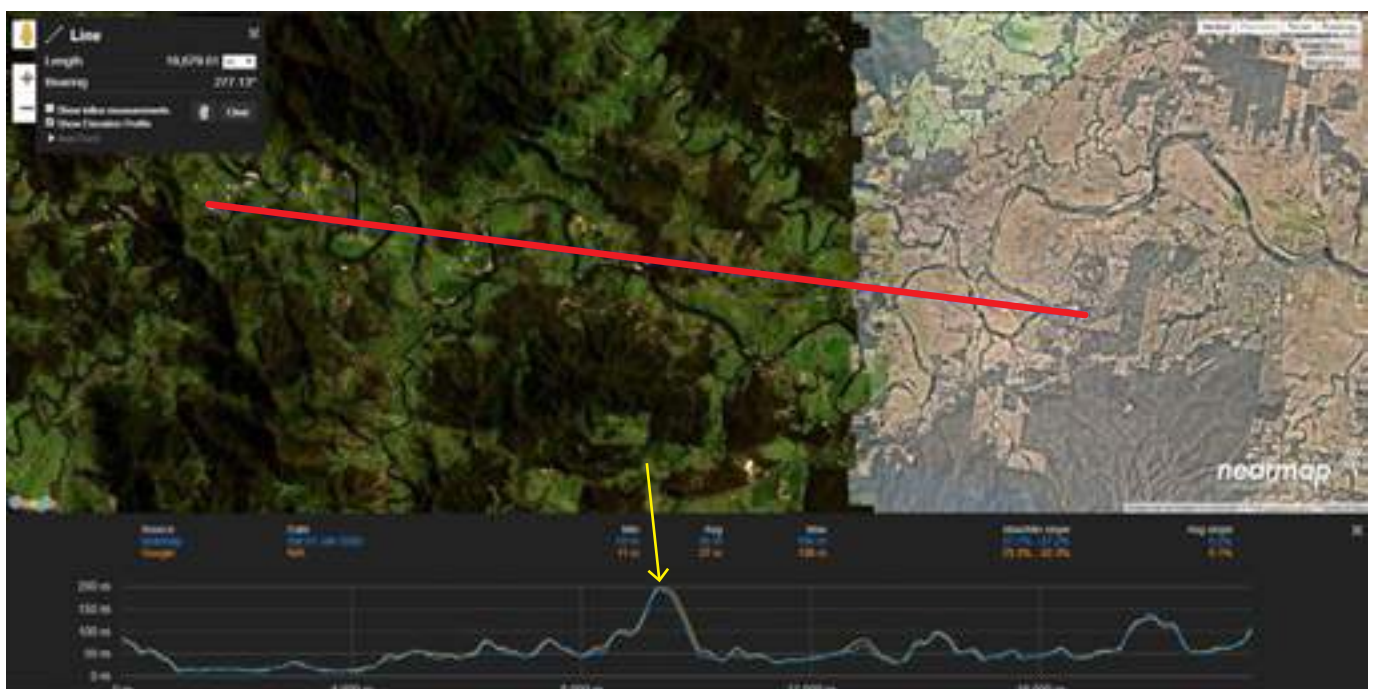
Figure 3. Signal path from Wauchope to Long Flat. The problem mountain range is shown with an arrow.
