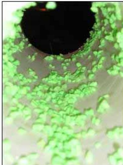
**Figure 4.4 Low to moderately tuberculated pipe model**
