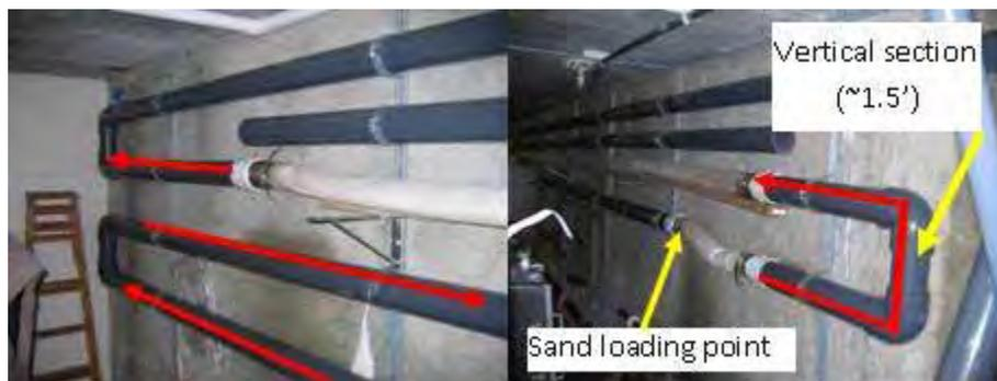
**Figure 4.1** Pipe loop used for flushing experiments
