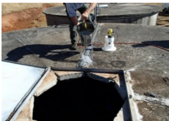
Figure 5: Bucket of Water Test
