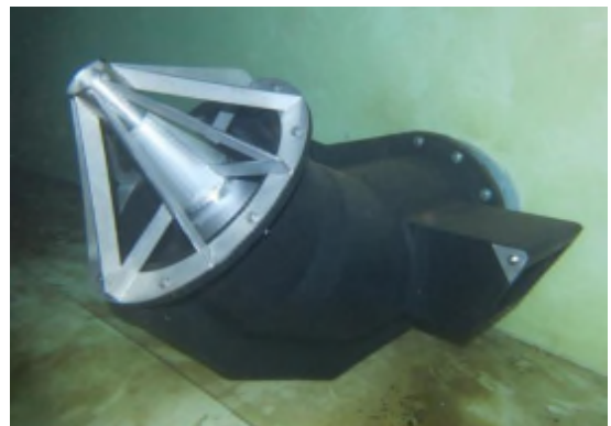
Figure 12: An Inlet Nozzle Directing Water Flow Up Off the Floor Area
