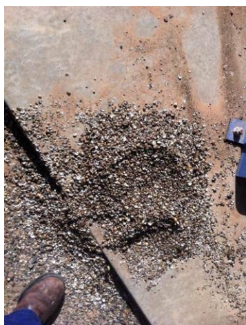
Figure 2: Shells and an Algae that usually clogs up the raw water pump's prefilter
