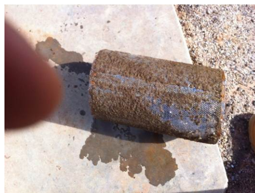
Figure 2: Shells and an Algae that usually clogs up the raw water pump's prefilter
