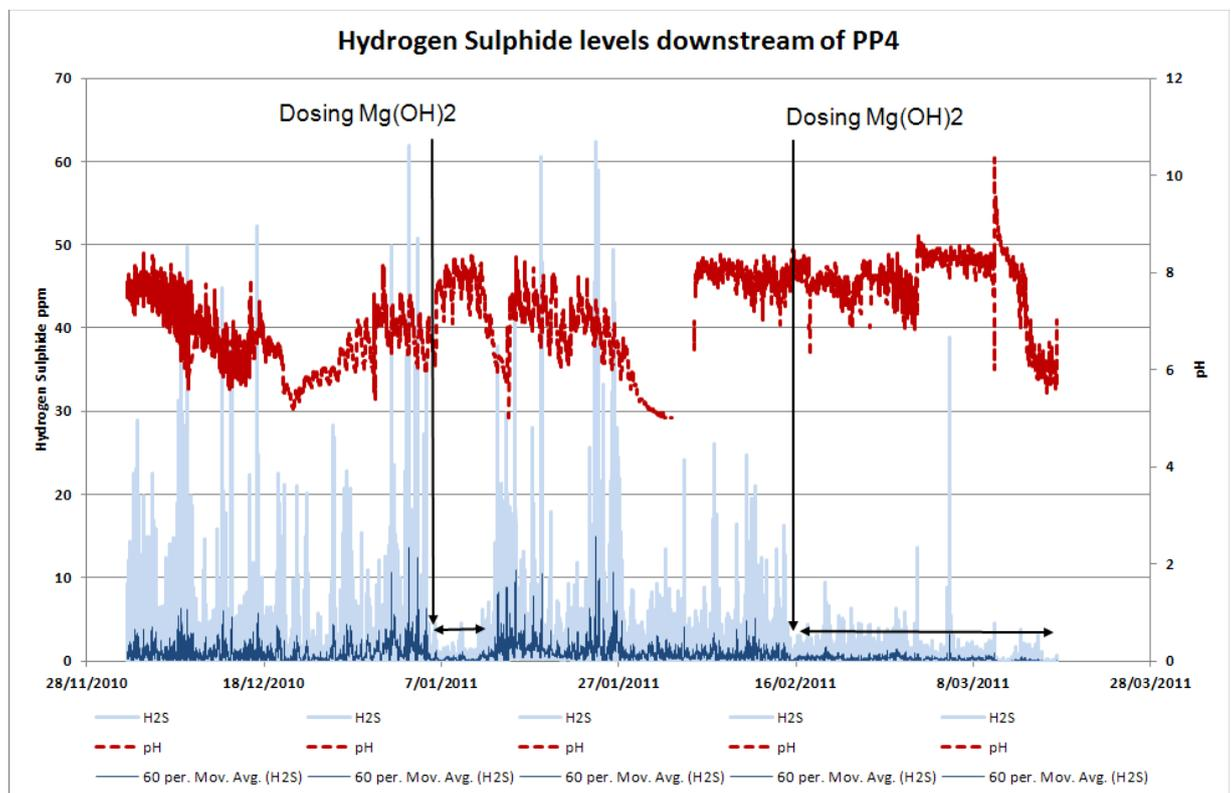
**Figure 3:** *Hydrogen Sulphide levels downstream of PS PP4*
