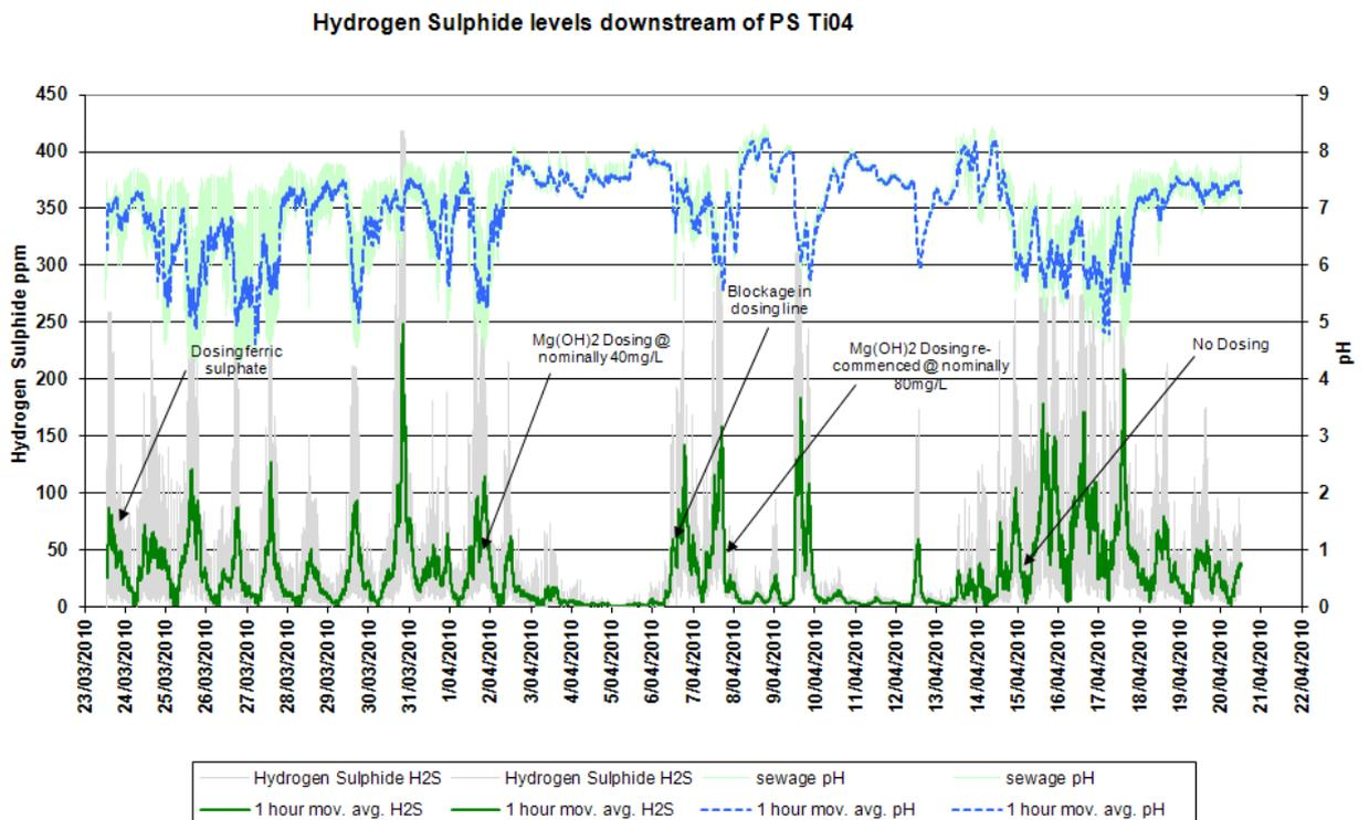
**Figure 2:** Hydrogen Sulphide levels downstream of PS Ti4
