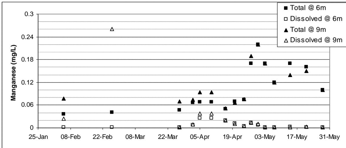
**Figure 3:** Manganese levels at Googong Dam offtake depths
