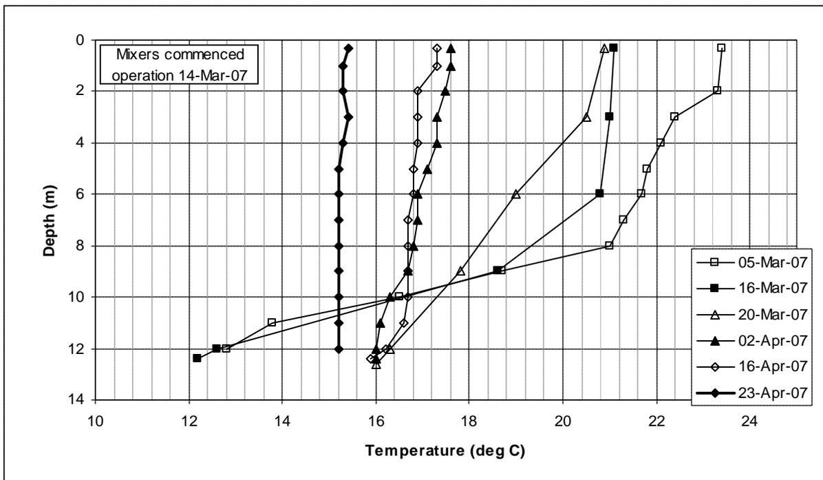
**Figure 2:** Temperature profiles at the Googong Dam offtake tower
