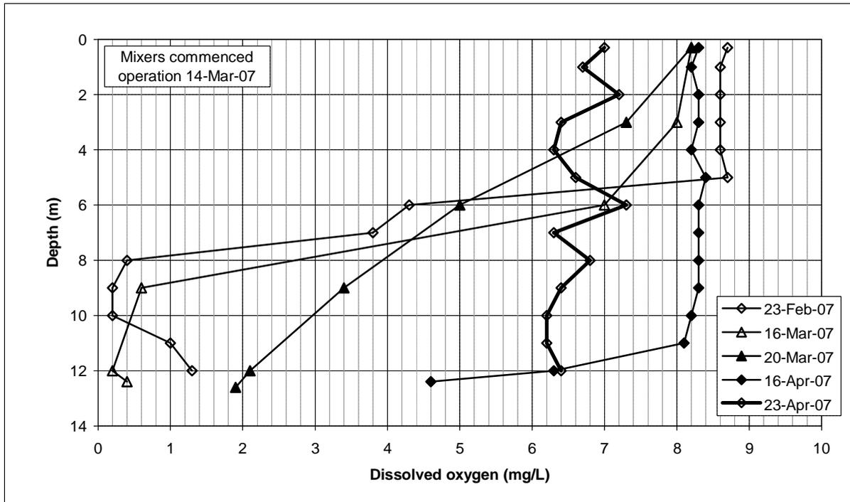
**Figure 1:** Dissolved oxygen profiles at the Googong Dam offtake tower
