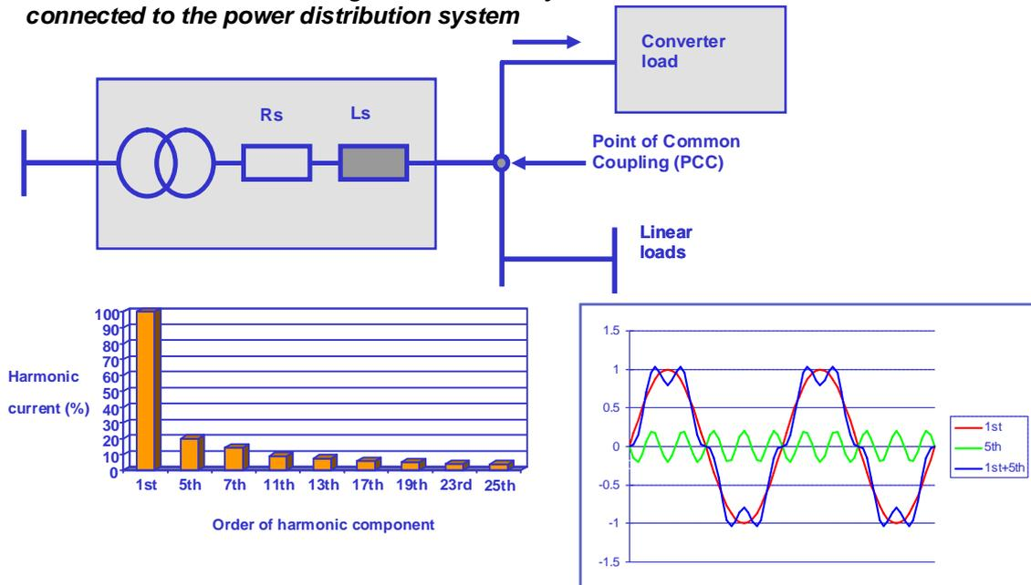
Other things to harmonic consideration are, the content of harmonic current can be affected by the construction of the variable speed drive, i.e. the level of inbuilt harmonic filtering. AC vs DC choke. The type of rectifier or IGBT rectifier, 6 pulse, 12 pulse or 24 pulse.
