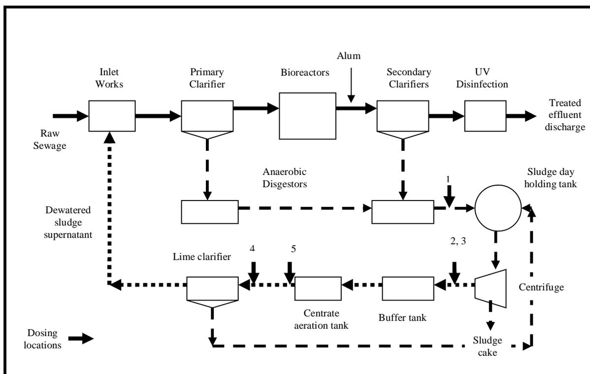
**Figure 1** *Process Layout of the Redcliffe WWTP*
